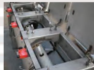
Hinged Cover with Safety Switches
